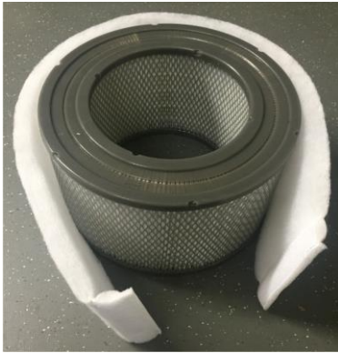
Fig. 4: Changing the prefilter
